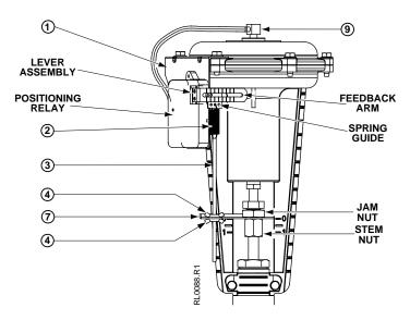
Figure 10. Positioning Relay Mounted on a Flowrite 599 Series 8-inch Valve Actuator.
