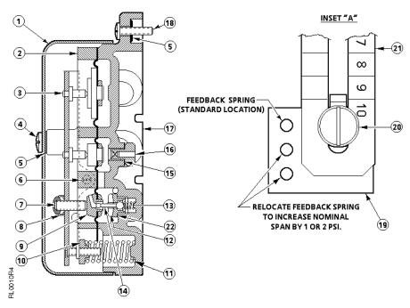
Figure 3. Construction of the RL 147 Positioning Relay.
