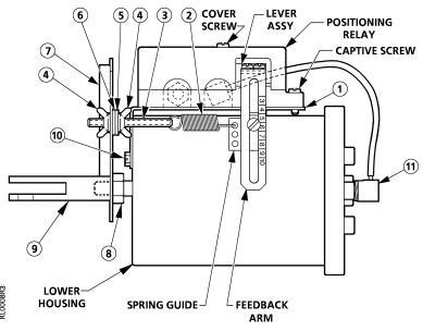
Figure 6. Positioning Relay Mounted on the No. 3 Damper Actuator.
