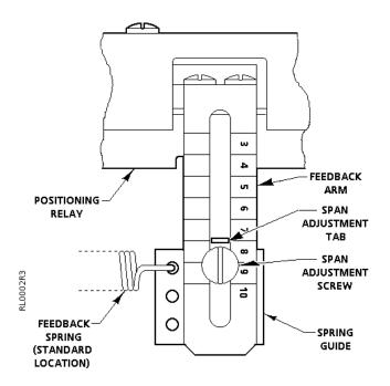
Figure 4. Span Adjustment. Shown at Span Setting 8.
